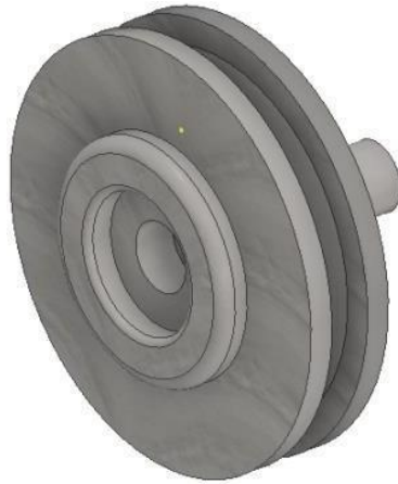
Fig.3. 11 Designed Magnetic wheel in Inventor
