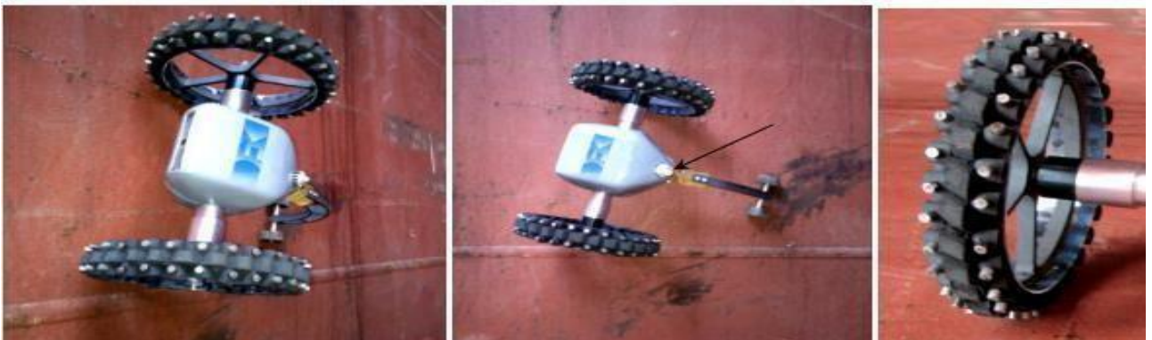
Fig.2. 15 A lightweight magnetic crawler with a designed magnetic wheel (Fondahl et al., (2012))
