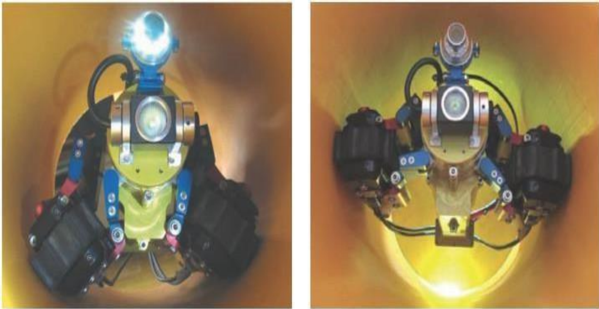
Fig.2. 8 Operational environments: a) horizontal pipe, \varnothing 235 mm, b) vertical pipe, \varnothing 235 mm (Ciszewski, et al., 2015).
