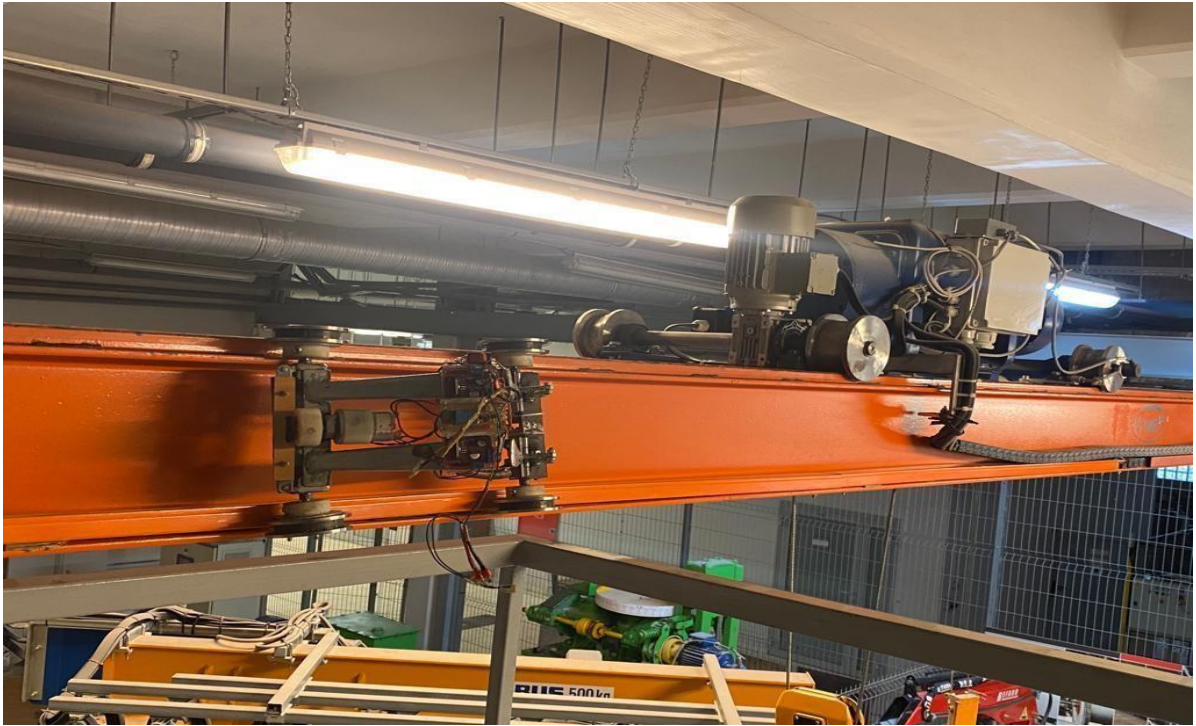
Fig.6. 26 (A) Movement of robotic tool on the vertical surface of overhead bridge
