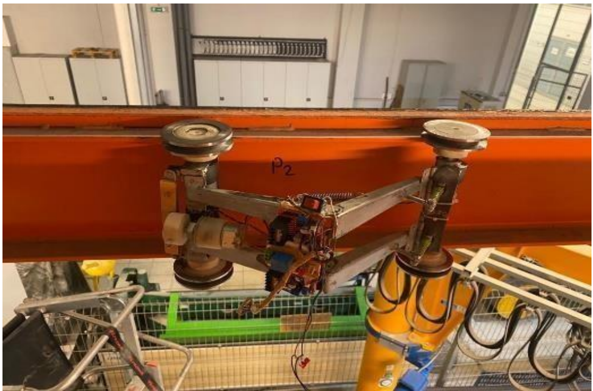
Fig.6. 26 (A) Movement of robotic tool on the vertical surface of overhead bridge
