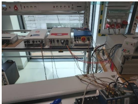
Fig. 5.11 Test bench for inverters
