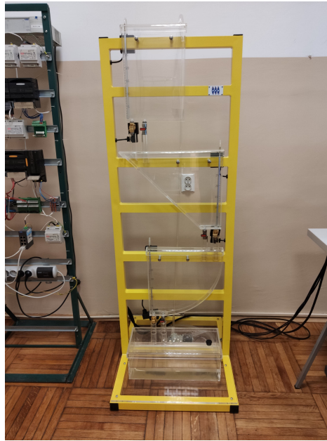
Figure 2.4: Photo of a system of three water tanks connected in a cascade. The entire system is connected to a computer that controls the pump and solenoid valves.
