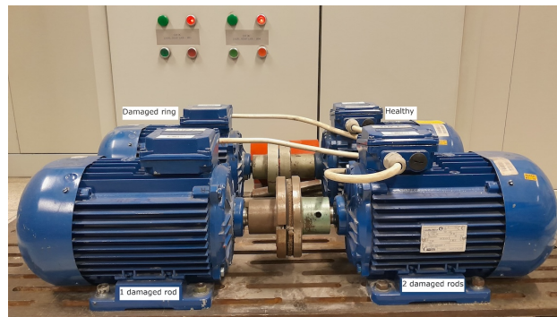
Figure 2.6: Setup of four motors used for data collection. One of them was healthy, and the rest was damaged in different ways: broken rotor bar, two rotor bars broken, broken end ring. In this analysis, we focused on the broken rod diagnostics.
