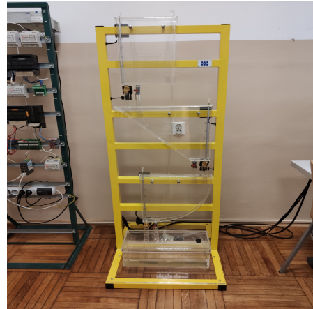
Fig. 1. Photo of a system of three water tanks connected in a cascade. the entire system is connected to a computer that controls the pump and solenoid valves.
