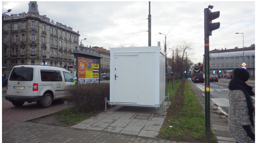
Figure 3. Example station used by the Main Inspectorate of Environmental Protection in their measurement system. The station name is Krakow, Dietla (code: PL0641A), and it is located near the city center and can measure the PM10 level, nitric oxide, nitrogen dioxide, and nitrogen oxides. Source: MIEP website [32].
